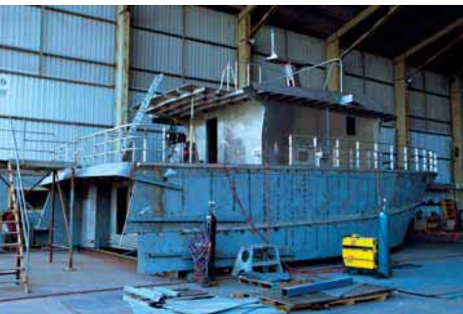
Adelaide Ship Construction - repairs and constructs boats for both commercial and private use. The company uses XLERPLATE® for the hulls of the vessels.
