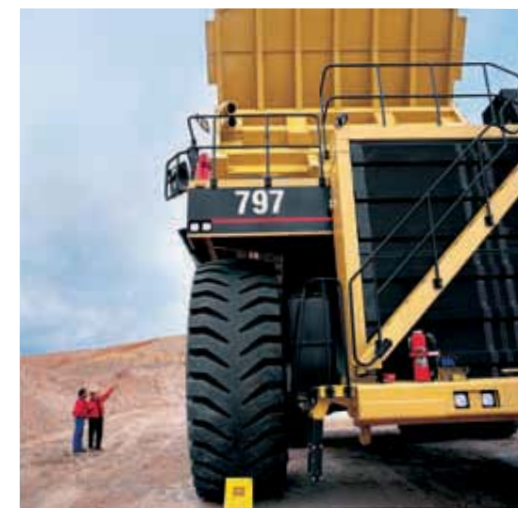
The Caterpillar Cat 797 (pictured left) is an Off Highway Truck locally built and designed for use in mining, with a maximum capacity of 326 tonnes and top speed (fully loaded) of 64 km/h.
